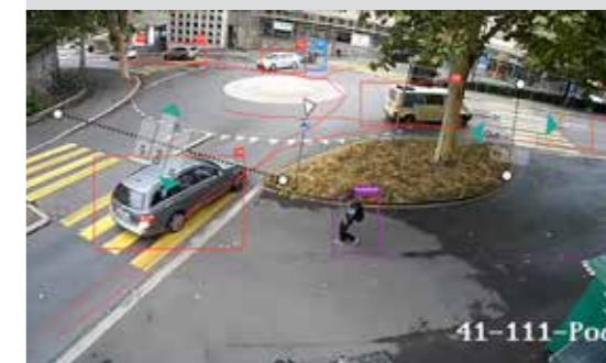
Automatic detection of traffic flow for all moving objects without storing video or image data.
