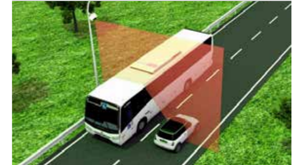
Two lanes can be covered simultaneously if the system is mounted at a height of around 8 m.
