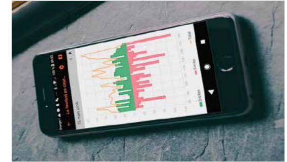
Automatic transmission of numerical data by LTE or SIGFOX. Counter visualisation on Android or iOS smartphones.
